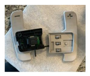
**Step 12:** Place the new paddles on the steering wheel and re-assemble the steering wheel. **MAKE SURE EVERYTHING IS CONNECTED BEFORE YOU PUSH THE AIRBAG BACK INTO PLACE.**
