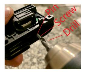
Using your drill, slowly engage the drill so that the self tapping screw digs into the spring pin just enough to hold it. Now using pliers, pull on the self tapping screw and pull the spring pin out of the paddle housing.
