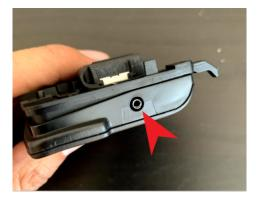
**Step 11:** Place the Touring, Formula, or Pro paddle on the OEM paddle housing and use the provided pin to connect both halves together.
