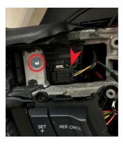
**Step 10 (Option 1):** Using the self tapping screws included with your order, line up the screw and insert it like the picture below.
