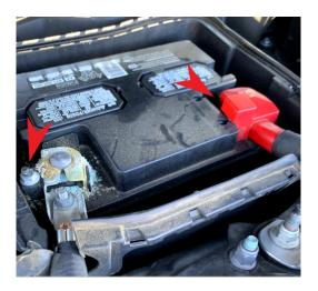
**Step 5:** Once the battery is disconnected and the terminals are in a good place, move to the inside of the vehicle.
